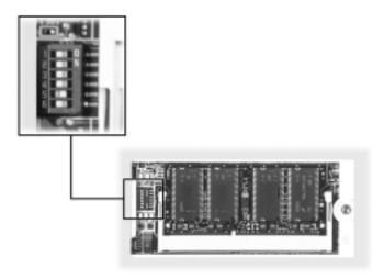
Note The system memory expansion slot is also located here. Therefore, if you need to install/replace SO-DIMM modules, you might want to do so when the system is already disassembled.
